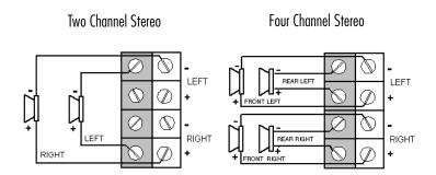
IOTE: For bridged two channel operation as shown in this diagram, connect right channel RCA cables to the front inputs of the amplifier, and left channel RCA cables to the rear inputs of the amplifier. For summed subwoofer applications, connect RCA cables per the input jack marking.
